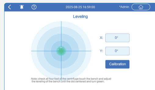
Electronic level assists in installation and leveling, making installation easier and simpler
